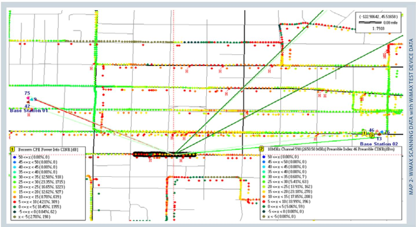
As can be seen, there is adequate signal level at this location for the POR011 sector with preamble index of 46 to be considered a valid neighbor. The systems engineers may consider changing the handover algorithm so that preamble 46 is considered a valid neighbor and remove the sector with preamble index of 80.
