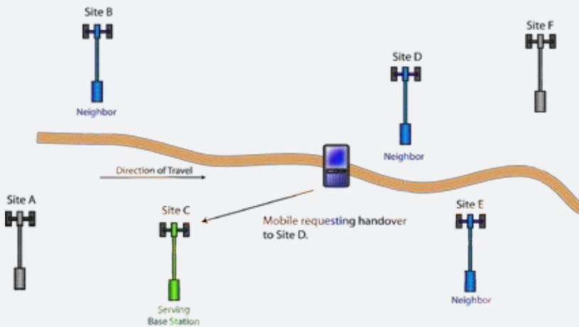
The mobile station evaluates the target base station(s) through previously performed scanning activity. The base station will respond with a base station handover response (MOB\_BSHO-RSP) message and the handover will commence when the mobile station sends the mobile station handover indication message (MOB\_HO-IND).
