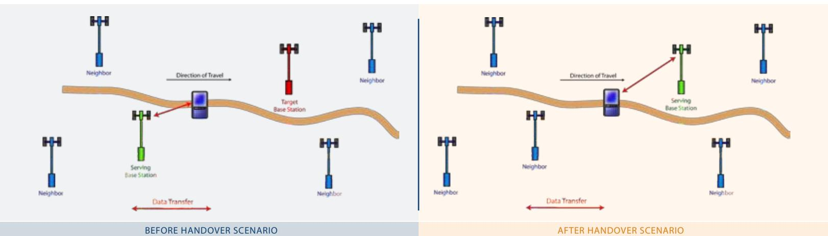
The network will define a signal quality threshold to trigger the handover when met. This may be a minimum CINR level, for example. When the mobile station's received CINR drops below the threshold, the mobile "hands-over" to the target base station. This involves a series of communications and messages that are beyond the scope of this white paper.
